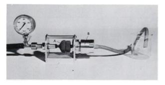
FIG. 2. In apparatus shown in Fig. 1 filter holder (A) containing filter is placed in position and ring B turned until gas-tight seal results. Cylinder tap is then slowly turned on until bubbles are observed in beaker. If premature bubbling occurs before given pressure is reached, there is defect in filter.
