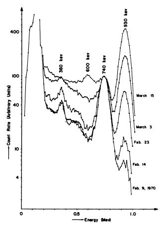
FIG. 1. Spectrum of <sup>90</sup>Mo obtained from alumina column (S ;uibb) at various time intervals.
