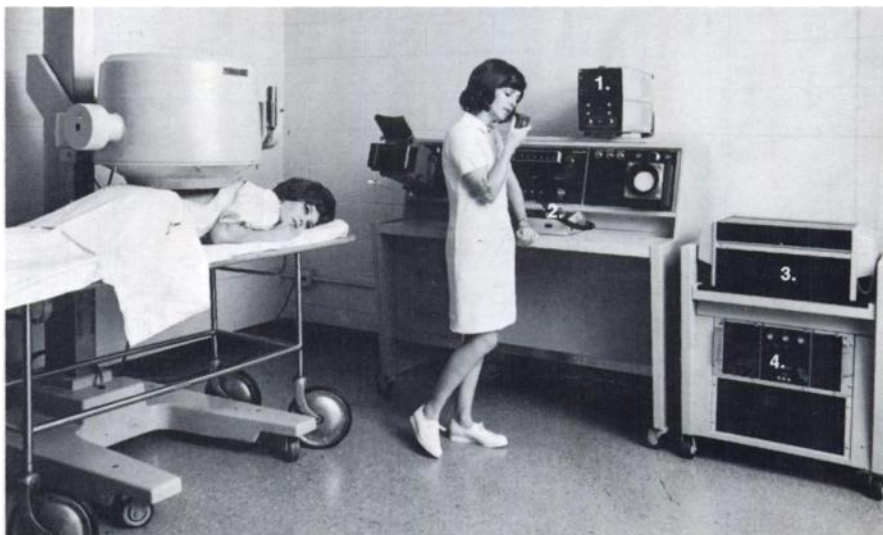
Components of the Data-Store/Playback Accessory: 1. Variable persistence oscilloscope. 2. Push-button control panel and microphone. 3. Data recorder. 4. Desk-height console for housing the data recorder and the required electronics.
