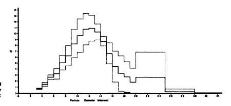
FIG. 1. Particle-size distribution of <sup>som</sup>Tc-tagged iron hydroxide; mean of four preparations. Dashed lines represent ± 1 s.d. from mean distribution.
