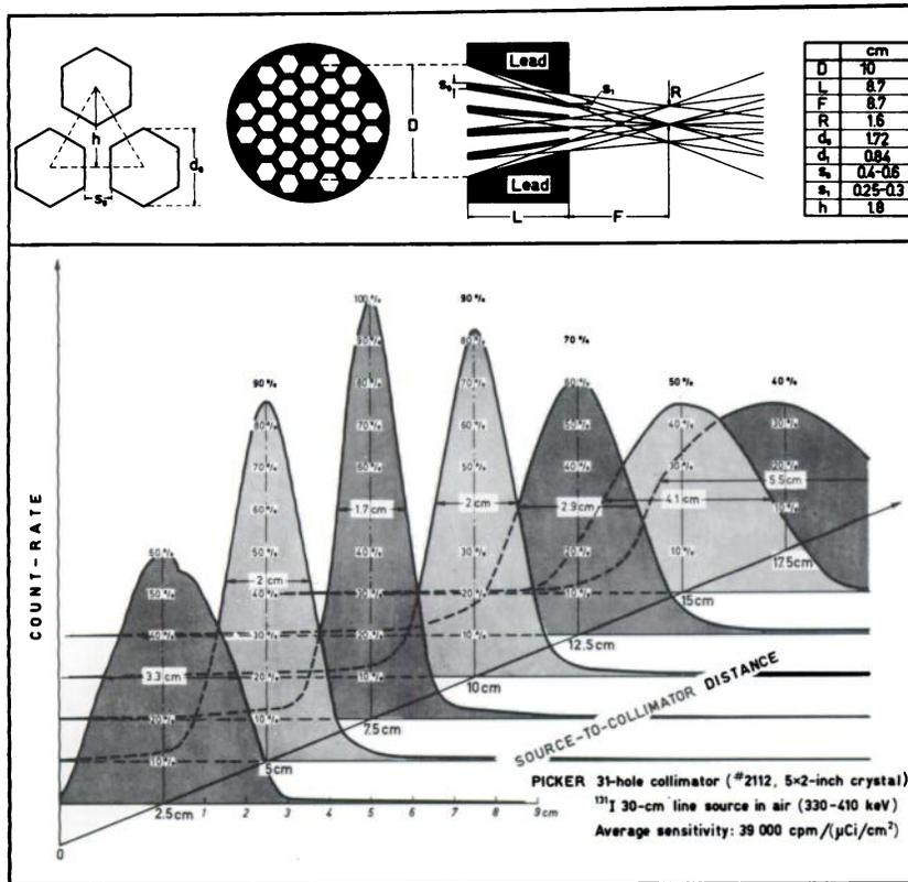
**FIG. 1.** Geometrical specifications of Picker #2112 collimator (top), and <sup>125</sup>I line-source response at 2.5-cm intervals from face of collimator (bottom).
