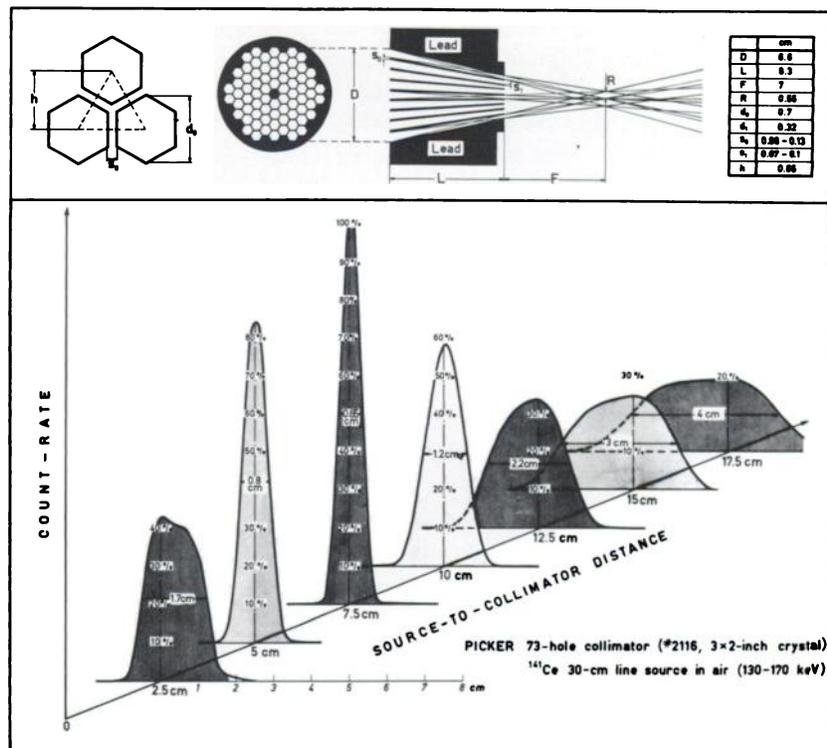
**FIG. 2.** Geometrical specifications of Picker #2116 collimator (top) and <sup>141</sup>Ce line-source response at 2.5-cm intervals from face of collimator (bottom).
