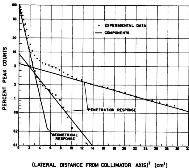
**FIG. 4.** <sup>131</sup>I line-source response of Picker #2107A collimator at 7.5 cm. Logarithmic plot of count-rate vs. linear plot of square of source distance from collimator axis. Experimental data can be analyzed into three straight-line components. Crosses represent data after subtraction of one component of penetration response; solid dots are data remaining after subtraction of both penetration response components.
