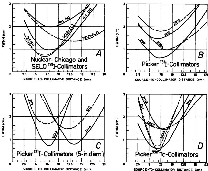
**FIG. 3.** Spatial resolution (FWHM) of 18 commercial collimators for various distances of source from face of collimator. A: Nuclear-Chicago and SELO 7.6-cm (3-in.-)dia  $^{131}\text{I}$ -collimators; B: Picker 7.6-cm (3-in.-)dia  $^{131}\text{I}$ -collimators; C: Picker 12.7-cm (5-in.-)dia  $^{131}\text{I}$ -collimators; D: Picker 7.6-cm (3-in.-) and 12.7-cm (5-in.-)dia  $^{99\text{m}}\text{Tc}$ -collimators.
