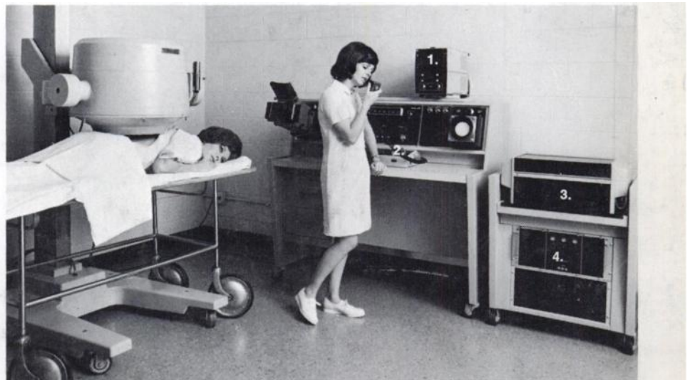
Components of the Data-Store/Playback Accessory: 1. Variable persistence oscilloscope. 2. Push-button control panel and microphone. 3. Data recorder. 4. Desk-height consolette for housing the data recorder and the required electronics.
