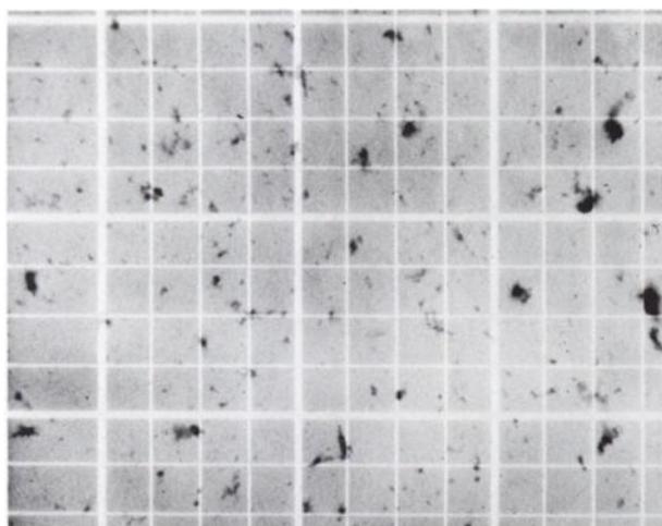
**FIG. 2.** Size of <sup>113m</sup>In-labeled particles prepared with iron carrier shown on a hemocytometer slide with light microscope. Majority of particles are in 1-5-micron range. Larger-appearing particles are aggregates of smaller-sized particles.
