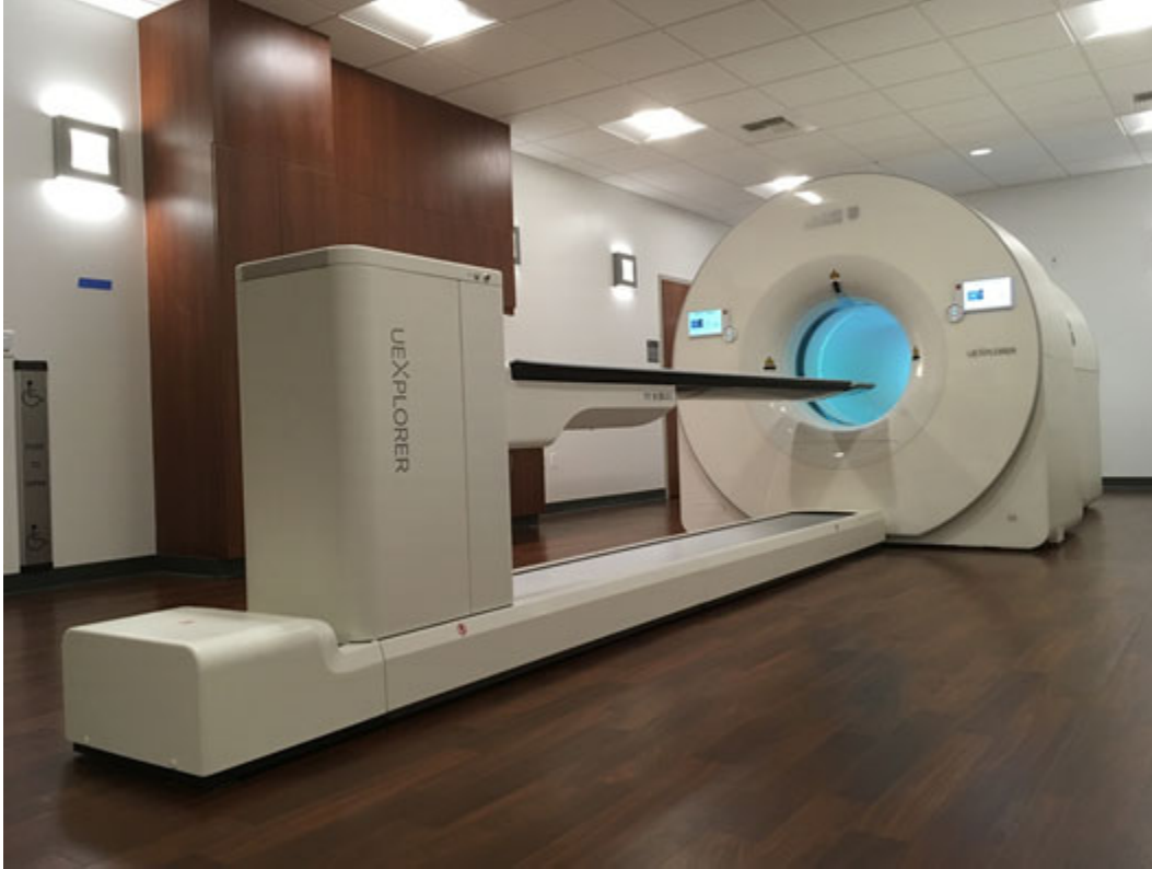
FIGURE 1. Photograph of the uEXPLORER total-body PET/CT scanner installed at the EXPLORER Molecular Imaging Center in Sacramento, CA, USA.
