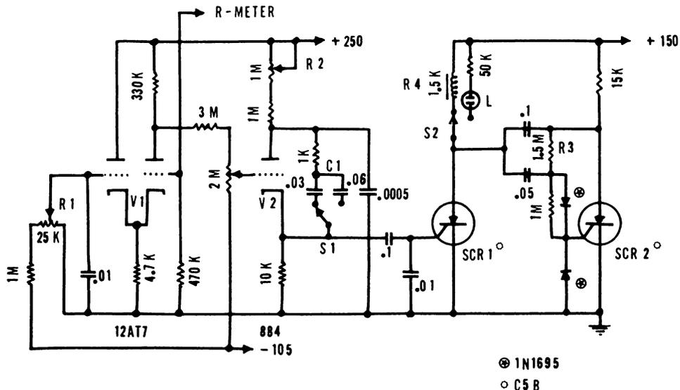
Fig. 1. Schematic circuit diagram of amplifier providing fixed background elimination, continuously variable proportional output, and an electronic print control switch.
