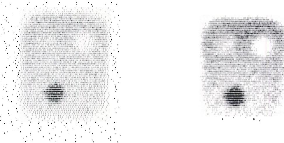
Fig. 3. Scans of phantom source containing iodine-131. Scan speed eight-inches per minute. Scan A *Left*: was recorded with a conventional scaled output, dot factor 1:16. Scan B *Right*: with the amplifier described (see text).  $C_M = 4500$  c/m;  $C_T = 1000$  c/m; time constant = 0.5 seconds.
