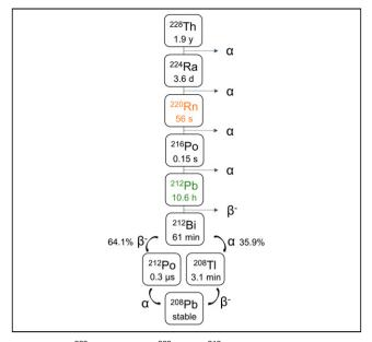
FIGURE 1. <sup>228</sup>Th series, with <sup>220</sup>Rn and <sup>212</sup>Pb highlighted.
