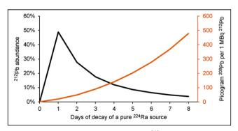
**FIGURE 3.** Relationship between radioactive <sup>212</sup>Pb and stable daughter nuclide <sup>208</sup>Pb as function of time, shown as abundance of <sup>212</sup>Pb relative to total amount of lead (black curve) and mass concentration of <sup>208</sup>Pb per 1 MBq of extracted <sup>212</sup>Pb (red curve), assuming generator yield of 62%.
