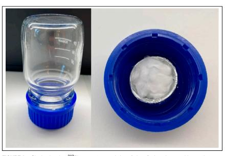
**FIGURE 2.** Single-chamber <sup>212</sup>Pb generator consisting of glass flask and removable cap that contains <sup>228</sup>Th or <sup>224</sup>Ra source fixed onto porous quartz wool.
