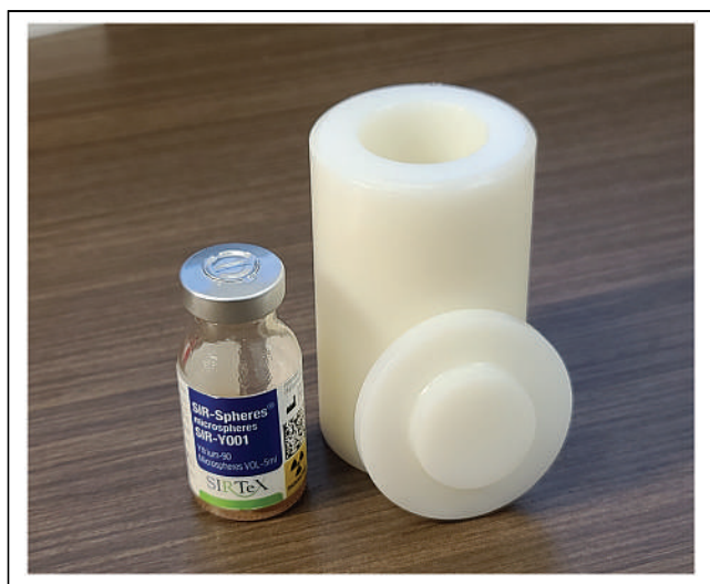
FIGURE 1. Photograph of custom high-density-polyethylene source holder and example SIR-Spheres patient vial.
