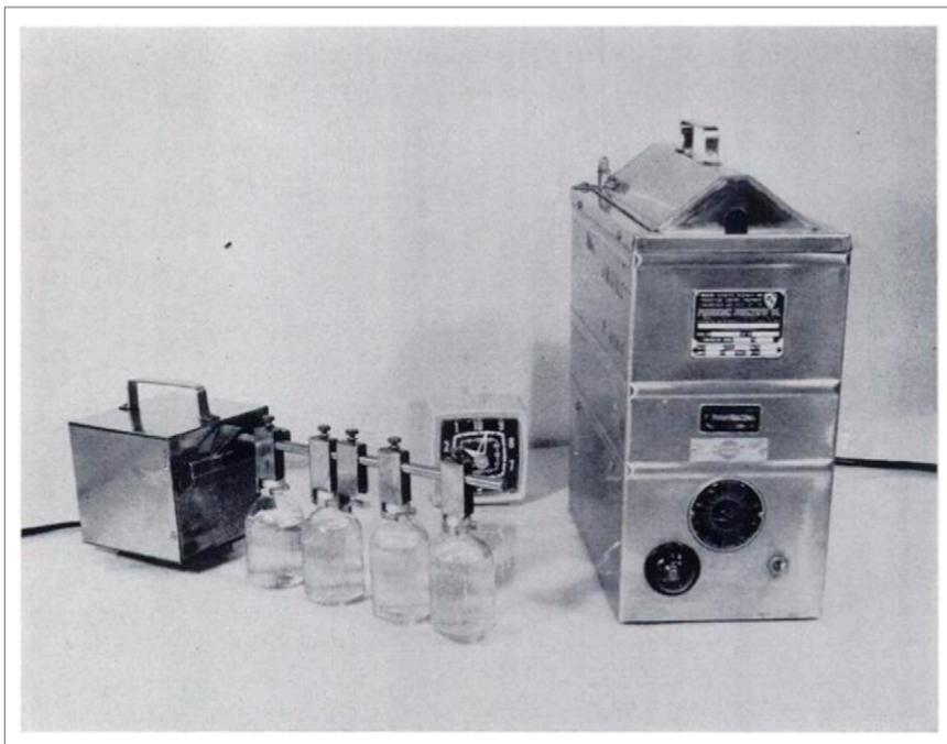
FIGURE 1. Motor driven sample shaker and precision water bath.
