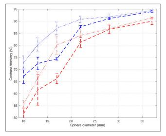
**FIGURE 4.** Contrast recovery and background variability measured with TOF OSEM – PSF (red lines) and Q.Clear (blue lines) at Stanford (dashed lines) and Uppsala (dotted lines).
