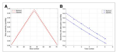
FIGURE 1. NEMA sensitivity measurements. (A) Sensitivity of different axial slices. (B) Sensitivity as function of number of attenuating aluminum sleeves.
