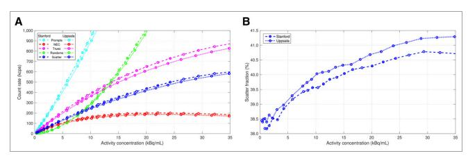
FIGURE 2. NEMA counting rate measurements. (A) Counting rate vs. activity. (B) Scatter fraction vs. activity. NEC = noise-equivalent counts.
