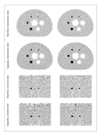
**FIGURE 5.** Image-quality phantom images reconstructed with TOF OSEM – PSF (left) and Q.Clear (right). Top two rows show transverse slices through center of all spheres. Bottom two rows show coronal slices through  $1^{9}_{13}$ -mm spheres.
