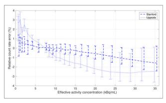
FIGURE 3. Counting rate error measured as percentage deviation from expected activity concentration. Error bars show range of deviations from expected activity level.
