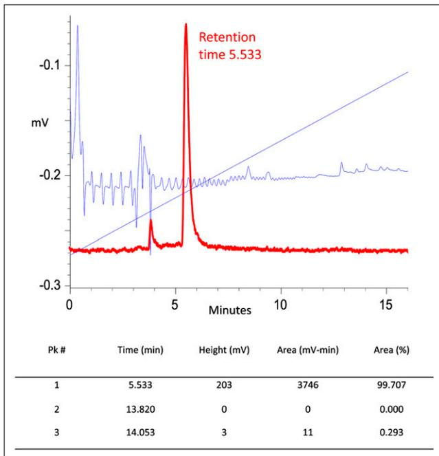
**FIGURE 1.** HPLC elution profile for  $^{64}\text{Cu}$ -TP3805. Radioactivity (99.7%) was eluted in single peak at retention time 5.53 min. Unbound  $^{64}\text{Cu}$  elutes at approximately 4 min. Diagonal line is percentage solvent gradient. Blue line indicates peptide ultraviolet elution; peptide mass injected was too small for ultraviolet detection. Pk # = peak number.
