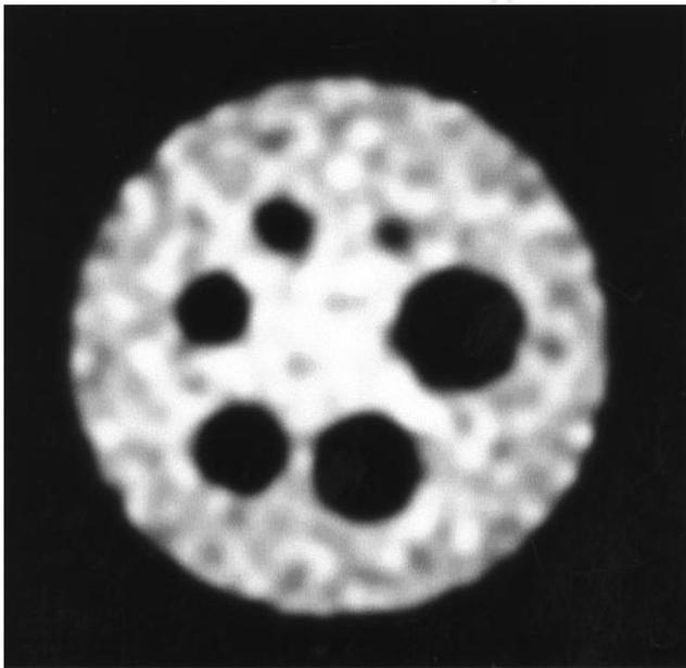
**FIGURE 5.** Transverse slice of cold spot phantom.
