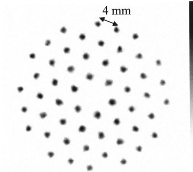
**FIGURE 2.** Transverse slice of multiple line source phantom.
