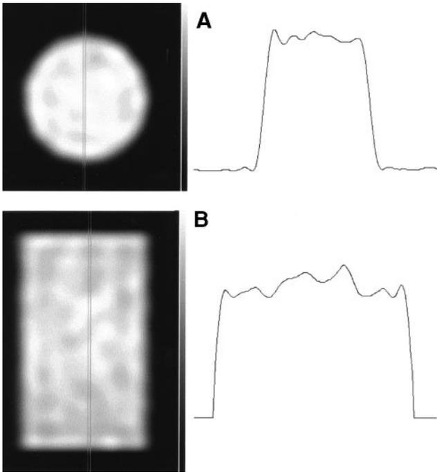
**FIGURE 4.** (A) Transverse slice of flood source phantom, with profile. (B) Coronal slice of flood source phantom, with profile.
