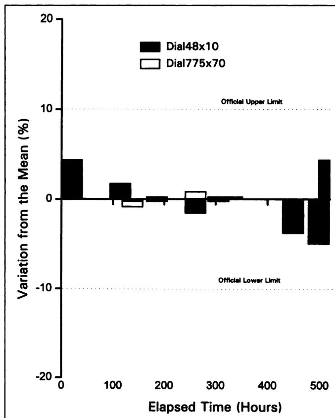
**FIGURE 1.** Capintec dose calibrator measurements (MBq) of  $^{90}\text{Y}$  from a linearity experiment at the 775  $\times$  70 and 48  $\times$  10 dial settings. The percent variations from the mean measurement ranged from -3.2% to +4.4% for the dial 775  $\times$  70 setting and -3.8% to +4.4% for the 48  $\times$  10.
