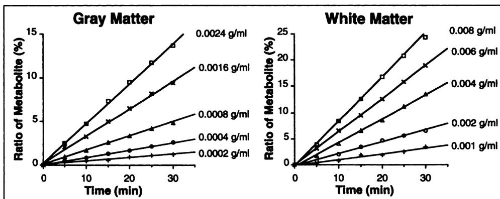
FIGURE 2. Temporal profiles of the ratios of metabolites in incubations with homogenates of cerebral gray matter and cerebral white matter of cynomolgus monkey. Data at 20–30 min in 0.008 g/ml white matter and data at 25 and 30 min in 0.006 g/ml white matter were not used in the analysis. The curves represent regression lines.
