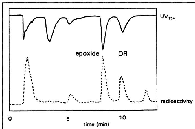
FIGURE 3. HPLC-radiochromatogram obtained for purification of  $^{11}\text{C}$ -daunorubicin.
