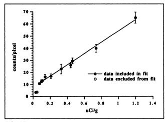
FIGURE 6. Phantom calibration. Two phantom studies were performed (see Methods) and the results were plotted: cts/pixel (ordinate) versus  $\mu$ Ci/cc (abcissa). A linear relationship was observed above 0.08  $\mu$ Ci/cc, but the line did not extrapolate through zero. Below 0.08  $\mu$ Ci/cc the curve appeared to be nonlinear. We limited our rough estimates of tissue radioactivity to ROI measurements of  $\geq$ 11 counts/pixel (~ $\geq$ 0.08  $\mu$ Ci/cc).
