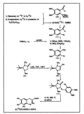
FIGURE 1. Radiolabeling of NCA 6-[<sup>18</sup>F]fluoro-L-dopa starting from its aryttrimethylammonium precursor.
