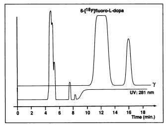
**FIGURE 3.** HPLC purification profile of 6-[<sup>18</sup>F]fluoro-L-dopa. Conditions: Whatman ODS 3 (7  $\mu$ ) column (9  $\times$  500 mm).
