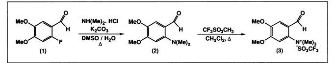
FIGURE 2. Chemical steps for the synthesis of the 6-trimethylammonium veratraldehyde triflate starting from 6-fluoroveratraldehyde.
