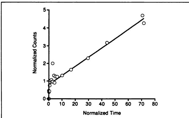
**FIGURE 3.** A linear fit of normalized time ( $[\int_0^t C_p^*(\tau) d\tau] / C_p^*(t)$ ) vs. normalized counts ( $C_i^*(t) / C_p^*(t)$ ) using a typical single pixel kinetic data set.
