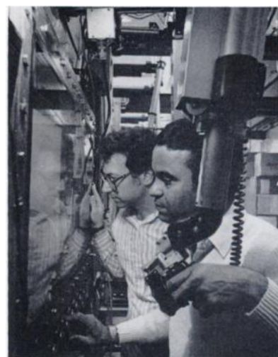
Suresh C. Srivastava, PhD (right), and Leonard F. Mausner, PhD, standing in front of the hot cell where radionuclides from the BLIP are processed. The targets are transferred from the BLIP by fork lift in lead casks which are connected to the hot cell through trap doors.
