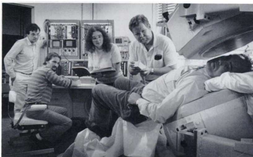
A. Bertrand Brill, MD, PhD, serves as a subject in the Universal Nuclear Imaging Construct (UNICON), a camera with flexible mounting and the capacity to detect both single-photon and positron emitters. Yves Bizais, MD, and George Zubal, PhD, observe from the console, while Wanda Rowe, PhD, takes notes and Gerry Bennett, PhD, positions the camera.
