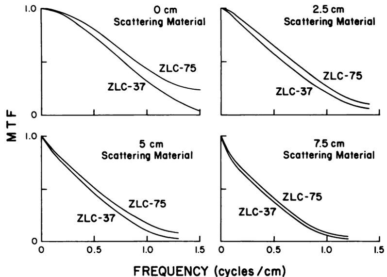
**FIG. 1.** Modulation transfer functions (MTFs) measured at various distances from collimator, using indicated camera, high-resolution, low-energy collimator, and 20% symmetric energy window. For all distances greater than 0 cm, region between collimator and source was occupied by tissue-equivalent scattering material. Note progressive diminution in difference in resolution between two cameras with progressive increase in distance from collimator.
