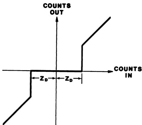
FIG. 2. Transfer function of operator at step (4) in Fig. 1.
