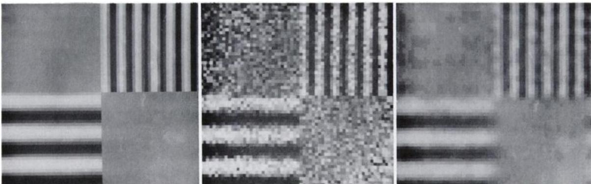
**FIG. 5.** Noiseless image (left). Count profiles across banded regions are sinusoidal. Same as left but containing noise (center). Final processed image (right). Regions of constant activity in Fig. 5(left) have minimal noise.
