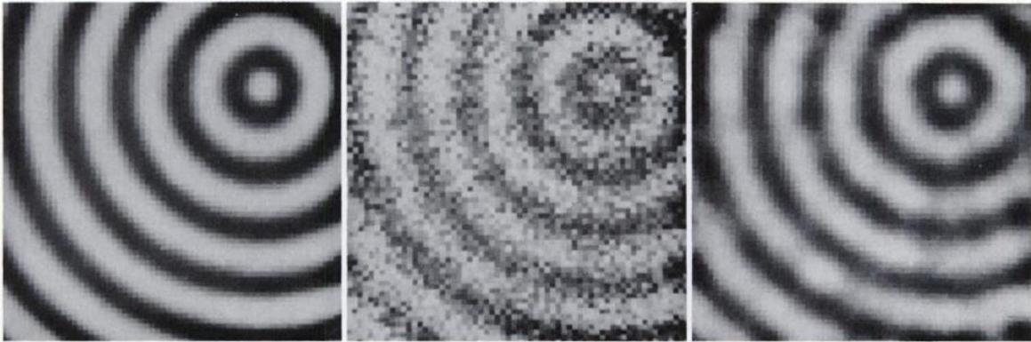
**FIG. 4.** Noiseless image (left). Count profile from center of bulls-eye radially is sinusoidal. Same as left but containing random noise (center). Final processed image (right).
