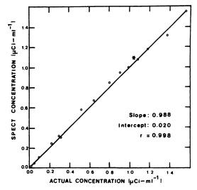
FIG. 1. Relationship between calculated SPECT concentration ( $\mu$ Ci/ml) and actual concentration of distributed extended source in a cylinder 22 cm in diameter. A constant calibration factor was determined using the Tc-99m 1.08  $\mu$ Ci/ml source.
