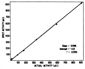
FIG. 2. Relationship between calculated SPECT-measured activity of point sources in air and actual activity ( $\mu$ Ci).
