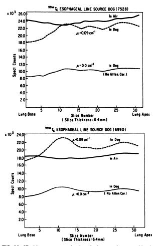
**FIG. 4A, 4B.** Line-source evaluations in dog esophagus and in air. SPECT counts obtained from ROI data are shown for each of 32 contiguous transaxial images. First and last slices correspond to lung base and apex. Value of  $\mu = 0.09$ /cm was used for attenuation coefficient with the first-order algorithm. Data indicated by  $\mu = 0.00$ /cm has not been compensated for attenuation. Note increased attenuation at lung base due to effects of heart and liver.
