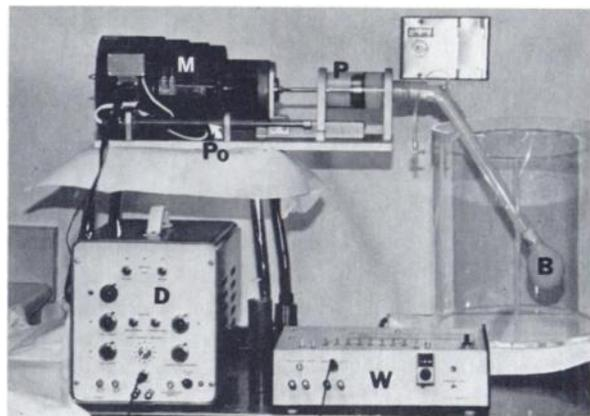
**FIG. 1.** B = balloon, P = pump, M = motor, Po = linear potentiometer, D = drive unit, W = wave generator.
