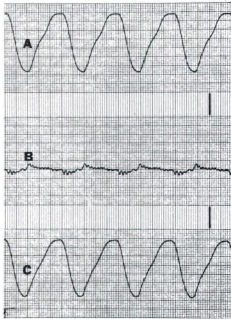
FIG. 2. Volumetric curves obtained at 60 cycles/min and 65-cc stroke volume. (A) Performance of the pump. (B) Difference between input signal and pump performance expanded four times. (C) Input signal from wave generator.
