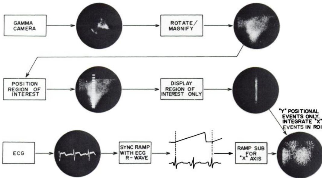
**FIG. 2.** Illustration of one method by which radionuclide kymograms may be generated. Gamma camera with region-of-interest (ROI) capability is used. The display is magnified and rotated to align the ROI. Only the vertical information from the ROI is used. Peak-detection circuit identifies R wave of ECG and triggers a ramp signal that sweeps the vertical profile across the scope as a function of time.
