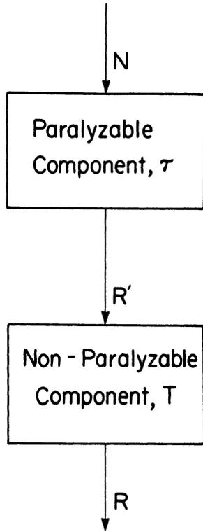
FIG. 1. Paralyzable-nonparalyzable counting system. Output of paralyzable component is input to nonparalyzable component.
