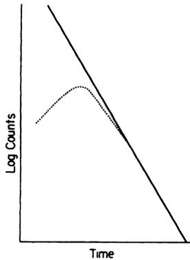
FIG. 2. Decaying-source method. Dotted line is R, recorded event rate. Solid line is Nw, the true event rate in window corresponding to the decay of Tc-99m.
