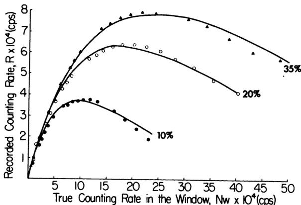
FIG. 4. Observed vs true event rates for Pho/Gamma IV camera at ● 10%, ○ 20%, and △ 35% window widths. Solid lines are data obtained from decaying-source method. Points are calculated from Eq. 5 using parameters in Table 1.
