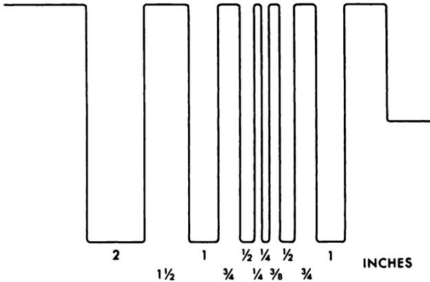
FIG. 1. Line spacing in phantom used for resolution studies.
