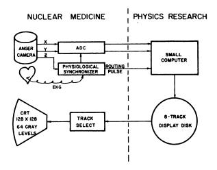
FIG. 1. Schematic representation of hardware configuration used for kinegraphic imaging.
