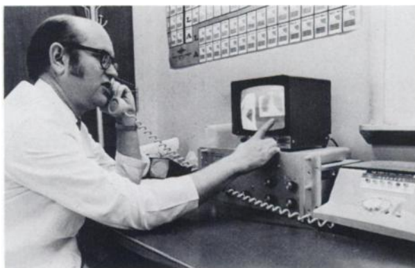
FIG. 1. Receiving terminal for nuclear medicine image communication system.
