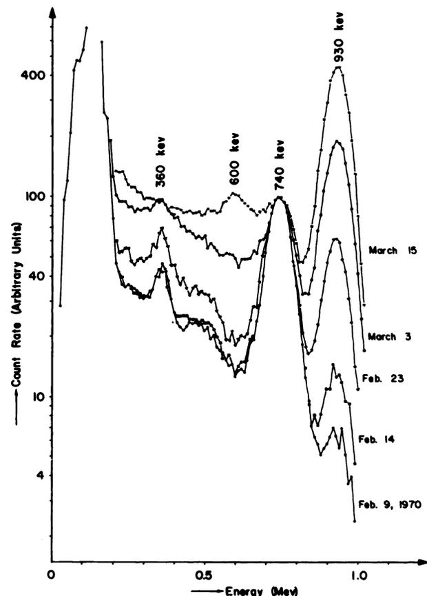
FIG. 1. Spectrum of  $^{99}\text{Mo}$  obtained from alumina column (Squibb) at various time intervals.
