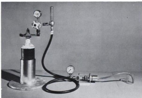
FIG. 1. Simple apparatus to test integrity of filters used for sterilization.
