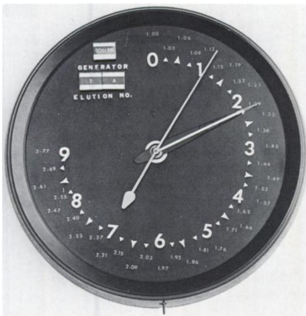
FIG. 1. Technetium-99m clock is constructed by removing ordinary numeral face from standard electric wall clock. Desired numerals are replaced using transfer lettering. Minute hand is removed because it is unnecessary, leaving hour hand to denote time increment. Second hand provides indication that clock is running properly. Identification magnets cling to steel face.
