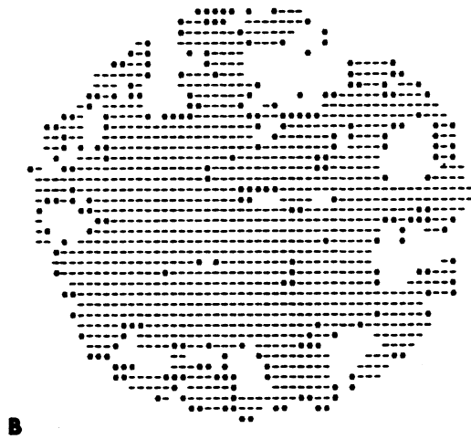
FIG. 2. A is photoscan of ^{131}\text{I} in phantom. B is three-level computerized plot of scan data gathered simultaneously with photoscan. Asterisks depict counting-rate increment that is 5% of maximum counting rate. Counting rates below this are represented by blanks and those above by hyphens. Two largest filling defects shown in Fig. 1 (right upper portion of photograph) are depicted at top of this scan.
