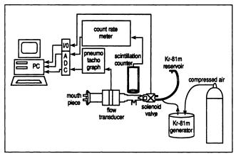
FIGURE 1. Schematic representation of the experimental setup. While seated in front of a LFOV gamma camera (not represented in the figure), the subjects breathe from the mouthpiece, while watching the computer screen.
