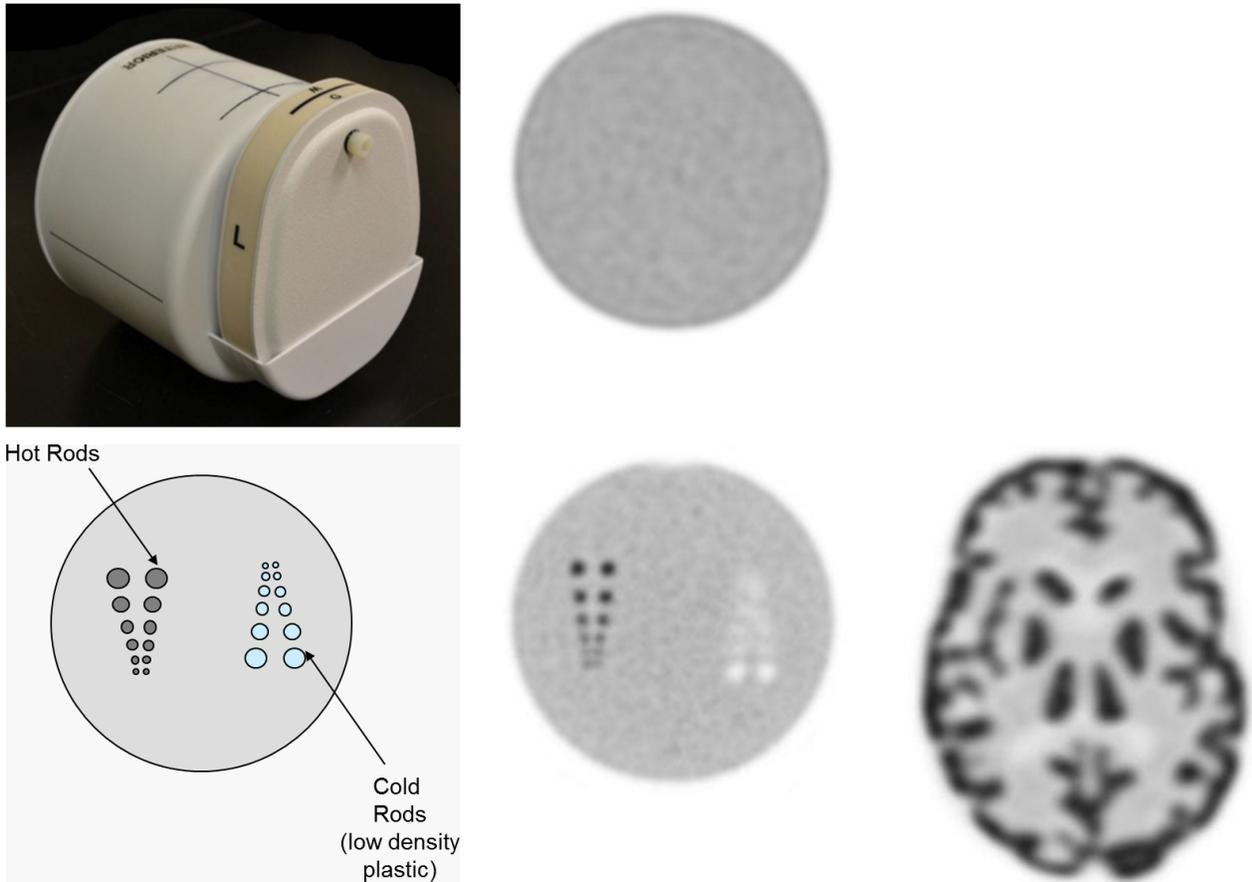
Figure 1. The SNMMI/CTN Qualification Phantom for PET Brain Imaging. A. Exterior of the phantom with the uniformity/resolution section to the left and the clinical simulation section to the right. B. Image from the uniformity section. C. Schematic of the resolution section. D. Image of the resolution section. E. An image of the clinical simulation section.
