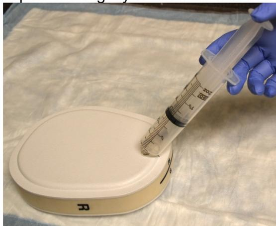
18. The G side of the phantom is filled with the dilute radioactivity from the Isopropanol bag. Use the large syringe to withdraw 50ml increments from the bag and inject into the G fill port. Repeat this process to completely fill the G side of the phantom with approximately 308 ml.
