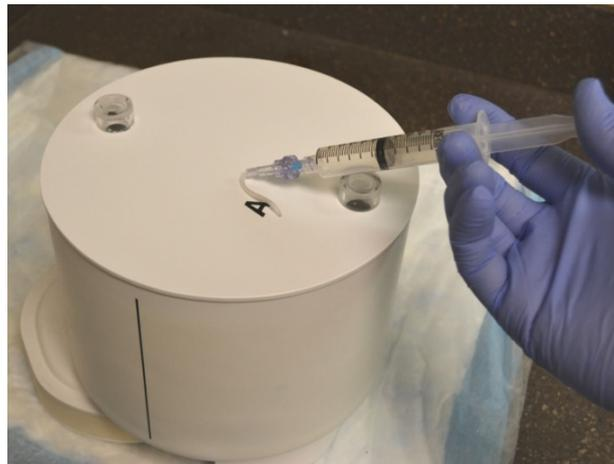
14. Remove the fill port screws and place the funnel into the one of the fill ports and add room temperature water (distilled water preferred if available) until filled (approximately 4,145 ml).
