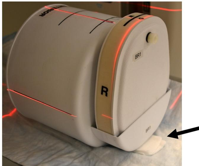
**Add padding to elevate the end of the phantom if necessary so that the phantom is aligned with the lateral lasers .**
