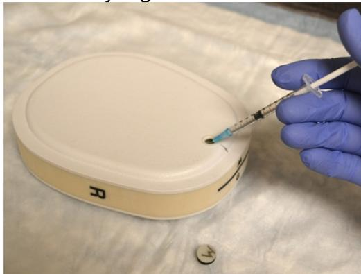
8. Place the short screw “W” in the W side fill port and secure. Gently rotate the phantom in several directions for 30 second to mix the radioactivity thoroughly.
