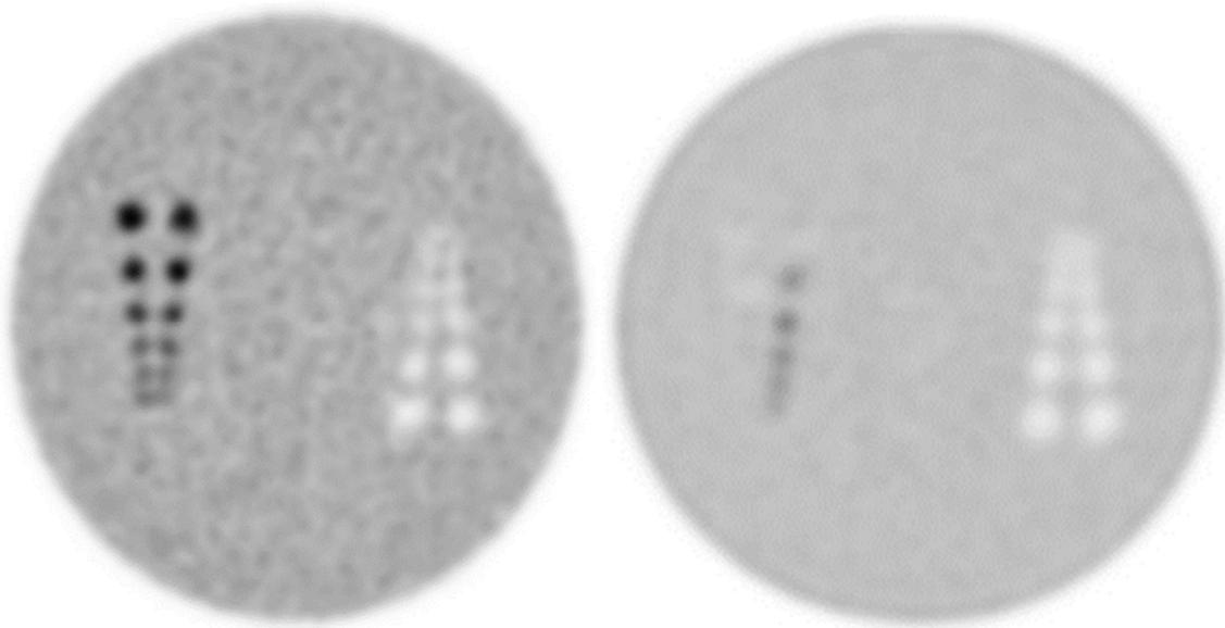
Figure 4. Images from the resolution section. A. Image with proper filling. B. Image with improper filling.
