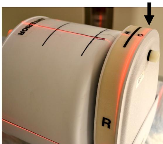
2. Once the phantom has been properly aligned select the brain protocol and perform the scout scan. Position the area to be scanned at the bottom of the clinical slab section of the phantom (arrow).
