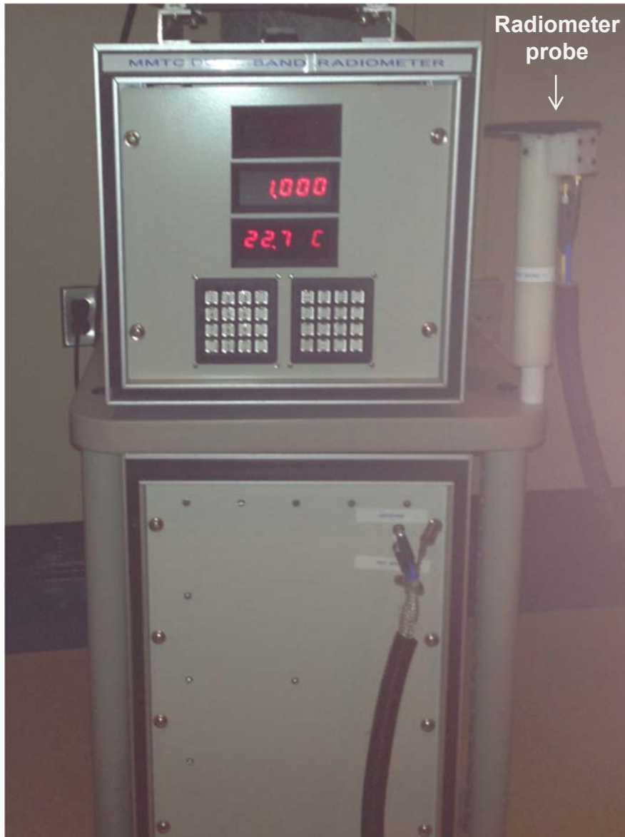
[Figure 1. Microwave radiometer system. This picture shows the microwave radiometry system used throughout the study. The probe used to collect radiometer data can be seen mounted on the right side of the picture.]
