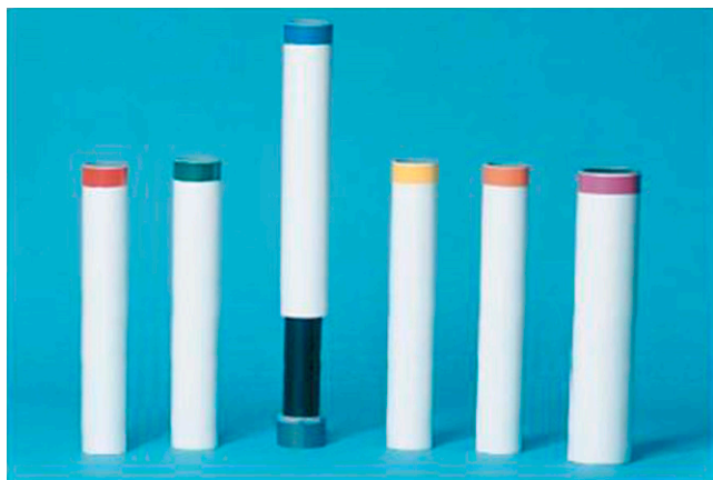
FIGURE 1. Set of lead-lined plastic sleeves (CalicheckDose Calibrator Linearity Test Kit; Fluke Biomedical) for evaluation of dose-calibrator linearity by shield method. Set is supplied with 0.64-cm-thick lead base, color-coded unlined sleeve (to provide activity measurement equivalent to 0 time point measurement of decay method), and 6 color-coded lead-lined sleeves providing attenuation factors nominally equivalent to decay over 6, 12, 20, 30, 40, and 50 h, respectively, for ^{99m}\text{Tc} .
