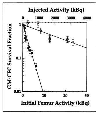
FIGURE 5. Survival of GM-CFCs as function of injected activity and extrapolated initial activity in femoral bone after intravenous administration of <sup>32</sup>P-orthophosphate (●) and <sup>33</sup>P-orthophosphate (○). Animals were killed on seventh day after injection, optimal day for GM-CFC assay (Fig. 4). SDs of mean for 3 independent experiments are shown.
