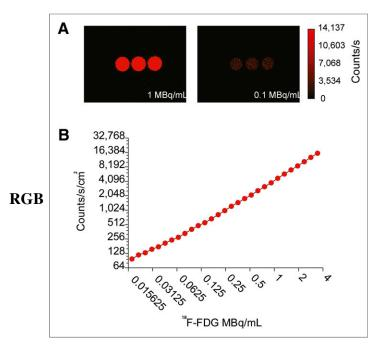
**FIGURE 1.** Sensitivity and linearity of intensified CCD to detect CL from <sup>18</sup>F-FDG. (A) CL imaging of multiwell plate with activity at 1 and 0.1 MBq/mL. (B) Linearity analysis of background-subtracted and decay-corrected region of interest of CL photon flux from wells using intensified CCD.
