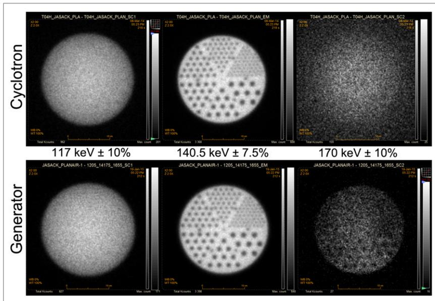
**FIGURE 5.** Typical phantom images obtained with cyclotron-produced (9 h after EOB; 723 MBq [top]) and generator-eluted (730 MBq [bottom])  $^{99m}\text{Tc}$ . Images are on linear gray scale, with white representing maximum intensity. Cold rods were 4.8, 6.4, 7.9, 9.5, 11.1, and 12.7 mm in diameter.
