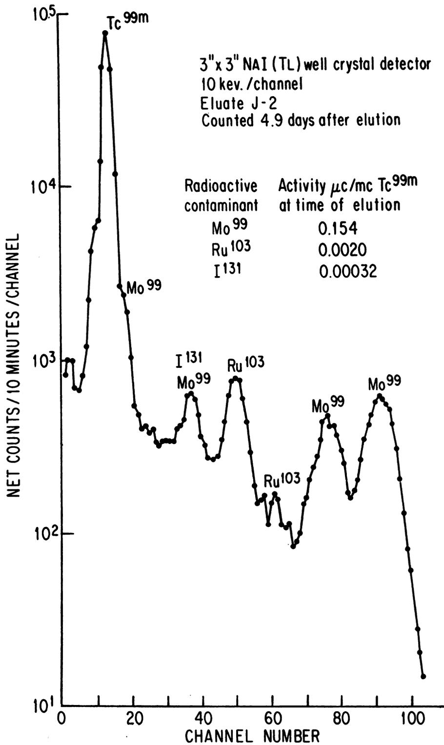
Fig. 4. Gamma-ray spectrum of an eluate from a  $\text{Tc}^{99\text{m}}$  generator illustrating photopeaks which can be identified as arising from radioactive contaminants.
