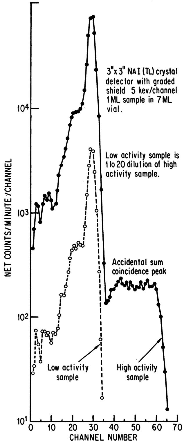
Fig. 5. Comparison of the gamma-ray spectra of high and low activity  $Tc^{99m}$  samples measured at 200 cm.
