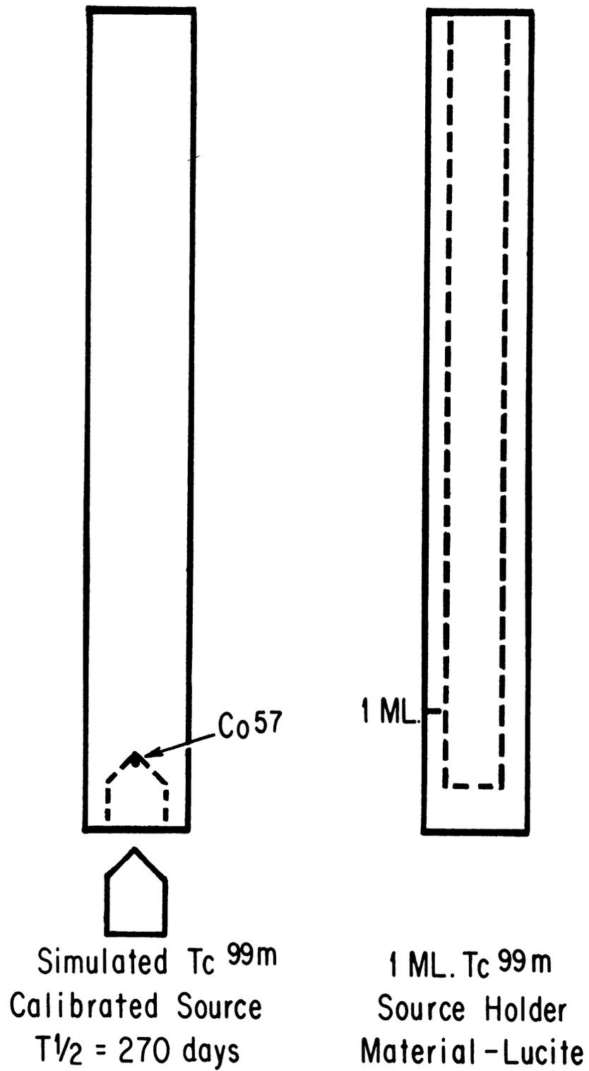
Fig. 6. Simulated Tc<sup>99m</sup> calibration source set.
