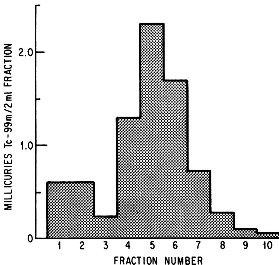
Fig. 3. Elution curve for a representative  $Tc^{99m}$  generator without the Dowex  $50 \times 8$  resin column.
