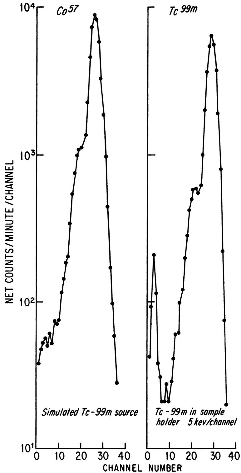
Fig. 7. Comparison of  $\text{Co}^{57}$  and  $\text{Tc}^{99m}$  gamma-ray spectrum in a NaI(Tl) well-crystal using the simulated  $\text{Tc}^{99m}$  calibration source set.
