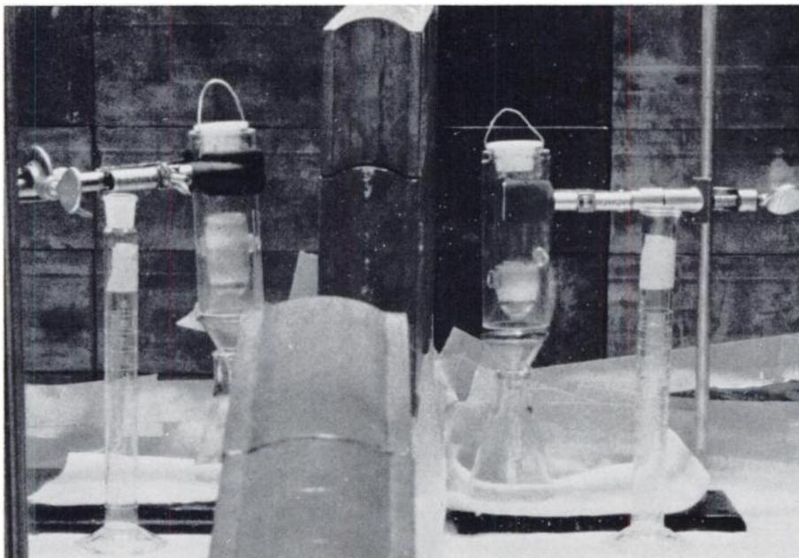
Fig. 2.  $Tc^{99m}$  generators in shielded enclosure. Generator on left has the Dowex  $50 \times 8$  resin column added.
