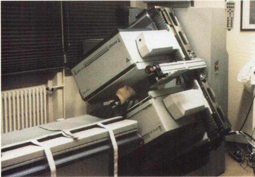
FIGURE 2. Prototype of conoscopic system was mounted on gantry without disturbing radial motion of heads.
