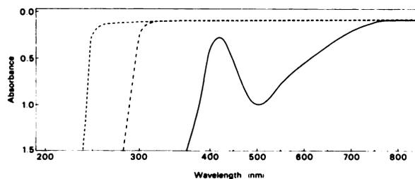
**FIG. 1.** Ultraviolet and visible spectra of various compounds in  $0.9\%$  NaCl at  $25^\circ\text{C}$ . Cuvette length: 10 mm. Reference: saline, —  $1.1 \times 10^{-2}\text{ M}$  Tc-99 glucoheptonate, .....  $0.07 \times 10^{-4}\text{ M}$  Tc-99 glucoheptonate, ---  $2.0 \times 10^{-2}\text{ M}$   $\text{SnCl}_2$  and  $1.0\text{ M}$  sodium glucoheptonate, - - -  $1.0\text{ M}$  sodium glucoheptonate.
