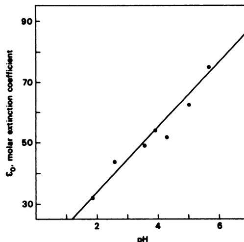
FIG. 4. pH dependence of the molar extinction coefficient at 502 nm of Tc-99 glucoheptonate (25°C).
