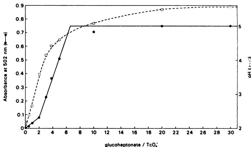
FIG. 3. Mol-ratio curve; absorbance at 502 nm (uv-vis. spectrum) and pH of Tc-99 glucoheptonate at different glucoheptonate to  $^{99}\text{TcO}_4^-$  ratios (25°C).
