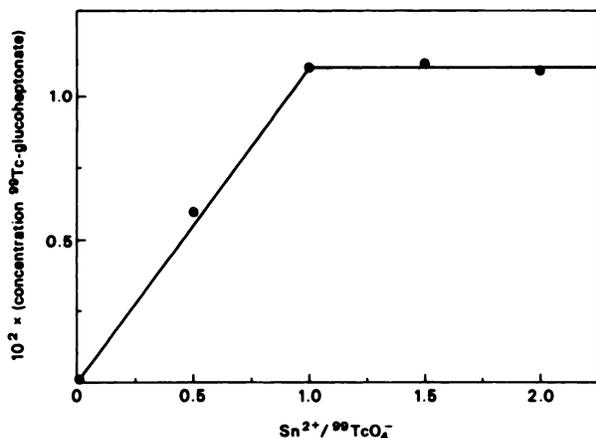
FIG. 2. Amount Tc-99 glucoheptonate formed at different molar ratios of Sn(II) and  $^{99}\text{TcO}_4^-$ , calculated from absorbance at 502 nm in the uv-vis. spectrum. Concentration  $^{99}\text{TcO}_4^-$ : 11 millimol in saline (25°C),  $\text{N}_2$  atmosphere.
