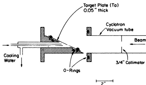
FIG. 1. Water-cooled target system used in production of K-38. About 100 mg of NaCl is deposited by slow evaporation on tantalum target plate in elliptical shape (axes 3.8 and 1.9 cm).
