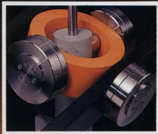
Gimbal suspension allows precise, swift and secure manual positioning of detector.
