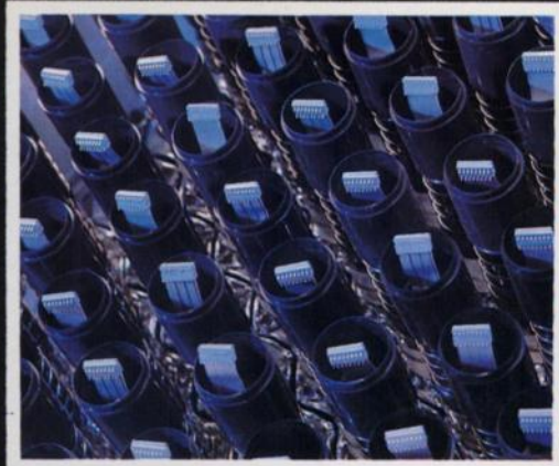
61 hexagonal "teacup" photomultiplier tubes produce superior resolution and linearity.
