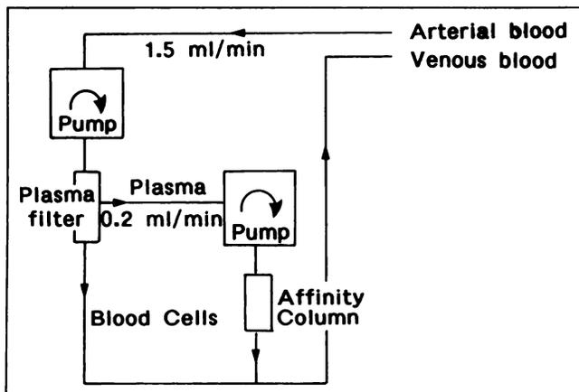
**FIGURE 1.** Experimental setup. Arterial blood is pumped at a flow rate of 1.5 ml/min through a plasma filter and plasma is pumped through the adsorbent column at a flow rate of 0.2 ml/min. After adsorption, blood cells and plasma are mixed and returned via an air trap to the vein catheter and back into the animal.
